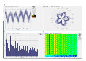
ZETLAB ANALIZ is a powerful set of instruments used for signals analysis (spectral, correlational, modal, order analysis, etc.)
